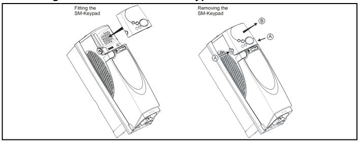
To fit, align the SM-Keypad and press gently in the direction shown until it clicks into position.
